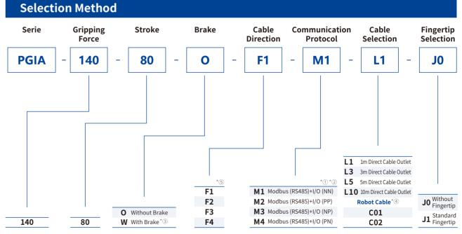
\*③When selecting a model with a brake, the gripper can maintain a certain gripping force after power-off, preventing materials from falling. "Power-off" here refers to cutting off the 220V power supply, at which point the gripping force will decrease to 85% of the powered-on leve
