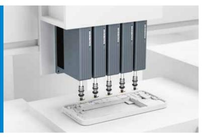
The product is compact, light, and thin. It employs a hollow rod design to support pick-and-place tasks. The intelligent soft landing function protects the picked and placed workpiece with precise force control. The Z-axis has a built-in spring to prevent the axis from
